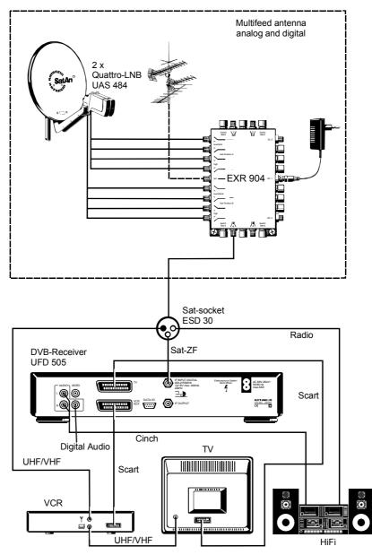
Connection of the DVB-S receiver to a TV set, a VCR and a hi-fi system for receiving and recording digital satellite TV and radio channels. The digital sound output can be connected to a Dolby Digital System.
